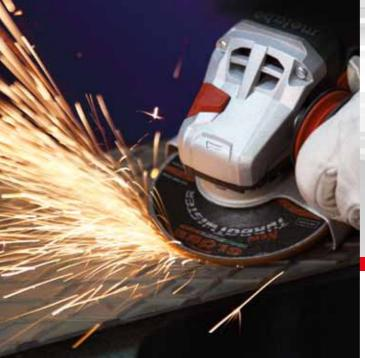
Turbotwister should be used at 15° angle with the working surface; this angle allows an higher contact area, the best finishing grade and more comfort.
